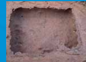
The wood in untreated plots is completely "eaten out" - only the mudding remains
