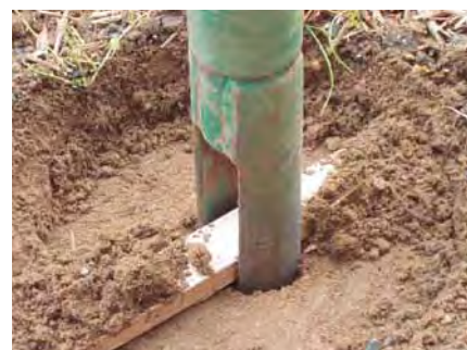
Picture 2: A piece of wood in the auger clearing the soil surface.
