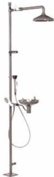
**Safety Showers and Eye Wash Fixtures** - Floor waste outlets in front of these fixtures dry out, allowing sewer gases to make their way into the habitable area due to lack of use, as the fixture is for emergency use only.
